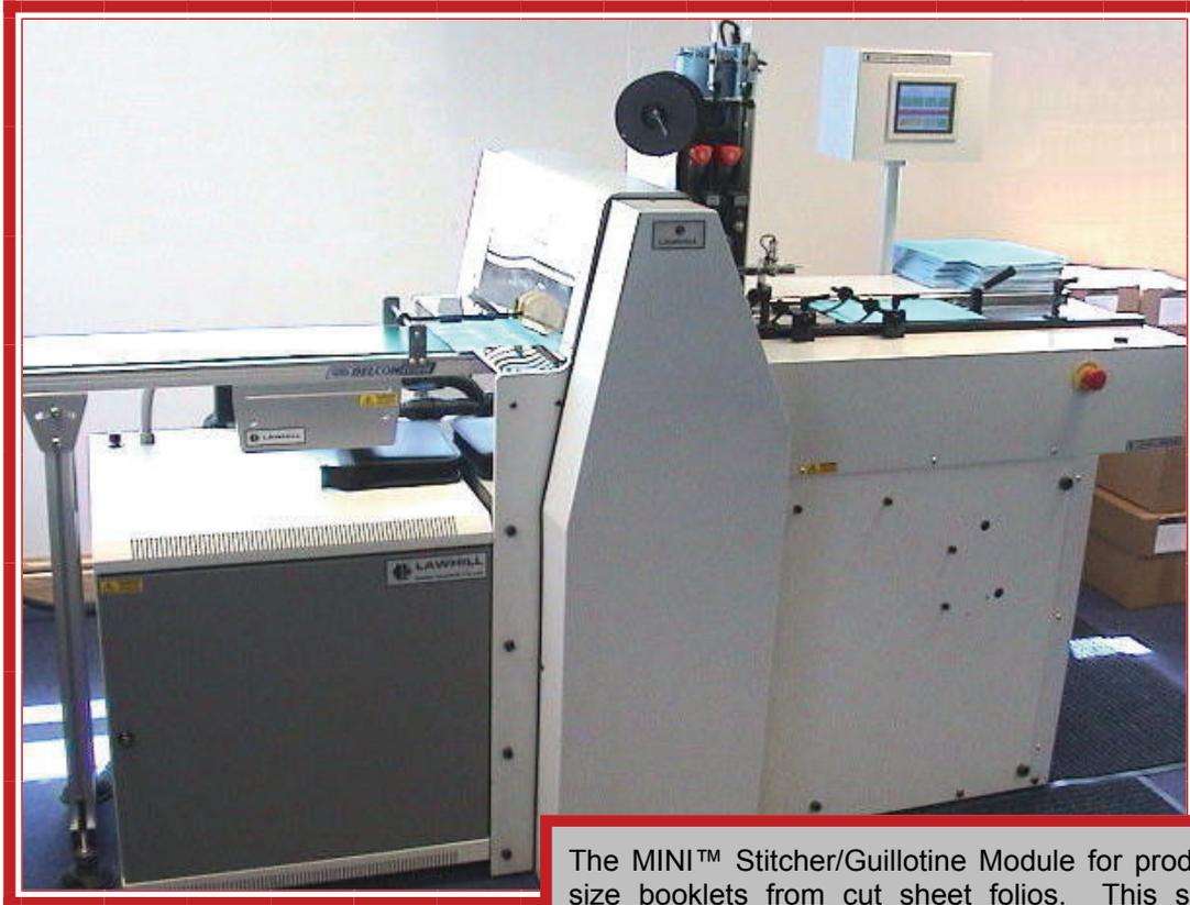
The MINI™ Stitcher/Guillotine Module for producing fixed size booklets from cut sheet folios. This system was designed specifically for the economic production of simple payment books up to 50 pages thick. Both units shown here have an integral output conveyor, but connection to other modules for binding or wrapping is also possible.
