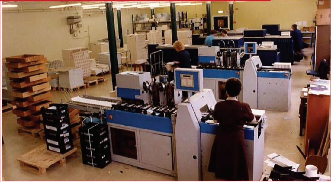
Typical production area showing the processing of 'Prestige' Stamp Booklets. The pre-printed four-to-view folios are first thread sewn in the fully automated Lawhill Sewing Module and are then passed to a **CHEKSAFE™** system for cutting and taping. This unit has been specially adapted to remove a gutter between each book, and to process two folios at the same time for greater productivity.
