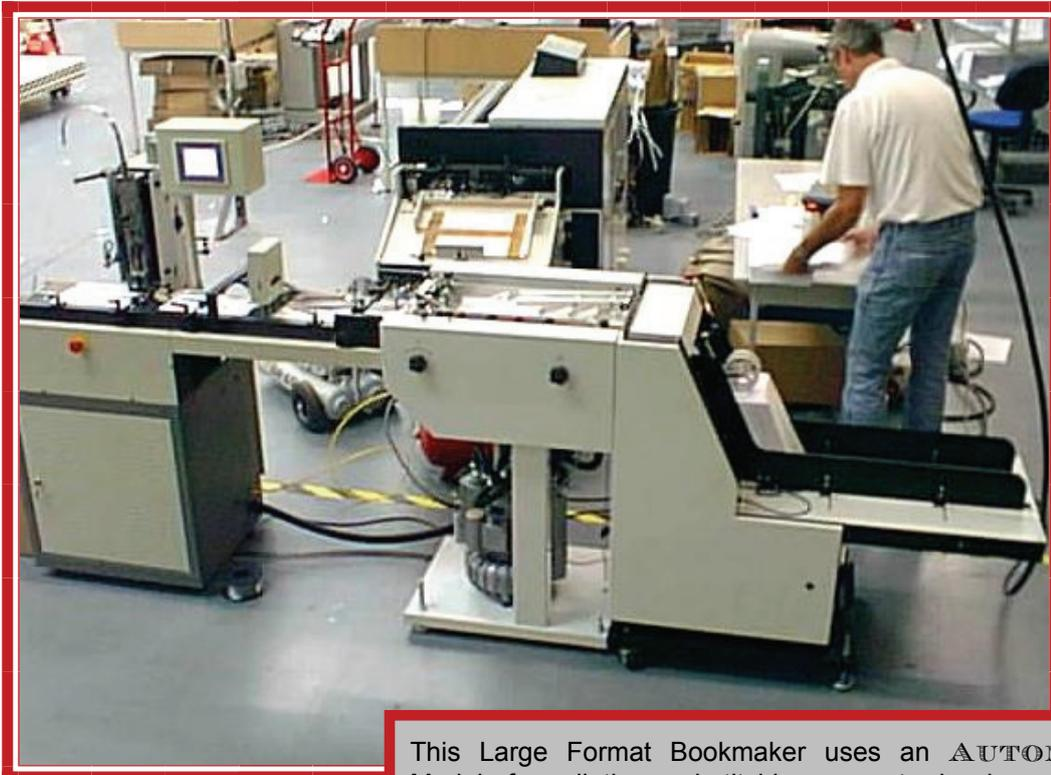
This Large Format Bookmaker uses an **AUTOMATE™** Module for collating and stitching computer hardware manuals. The verification is by both count and checking that the last sheet in each collation has a company logo correctly positioned.
